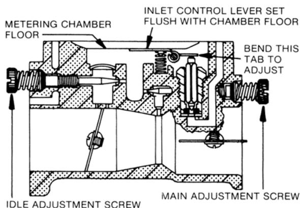
Be certain main diaphragm, gasket and cover casting are carefully fitted over the three small pins cast in rim at bottom of metering body; also the fuel pump gasket, diaphragm and fuel pump body, over similar pins at bottom rim of main diaphragm cover casting. Evenly tighten fuel pump body retaining screws to insure complete seal of casting separations at both diaphragms.
