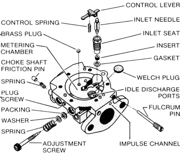
Control Lever must rotate freely on Fulcrum Pin. Set Control Lever flush with floor of metering chamber.
